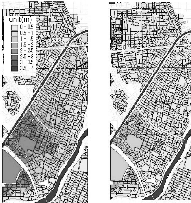
Figure 6. Computed inundation depth distributions at 3 h without pumping on the left and with the pumping of 30\text{m}^3/\text{s} on the right.
