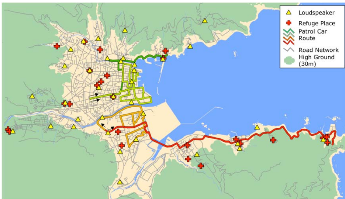
Figure 3. Owase's current warning transmission and evacuation facilities (35 emergency warning loudspeakers, 4 route alert vehicles, and 25 shelters, serving 6,651 households)
