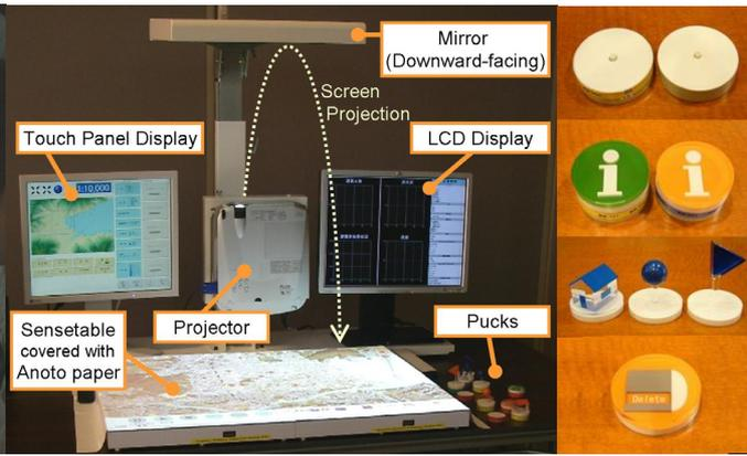
Figure 2. System architecture(left) and pucks(right).
